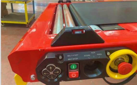
Front Control Panel
