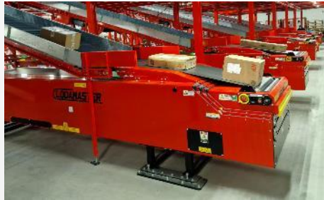
Raised Belt/Sliding Hood
