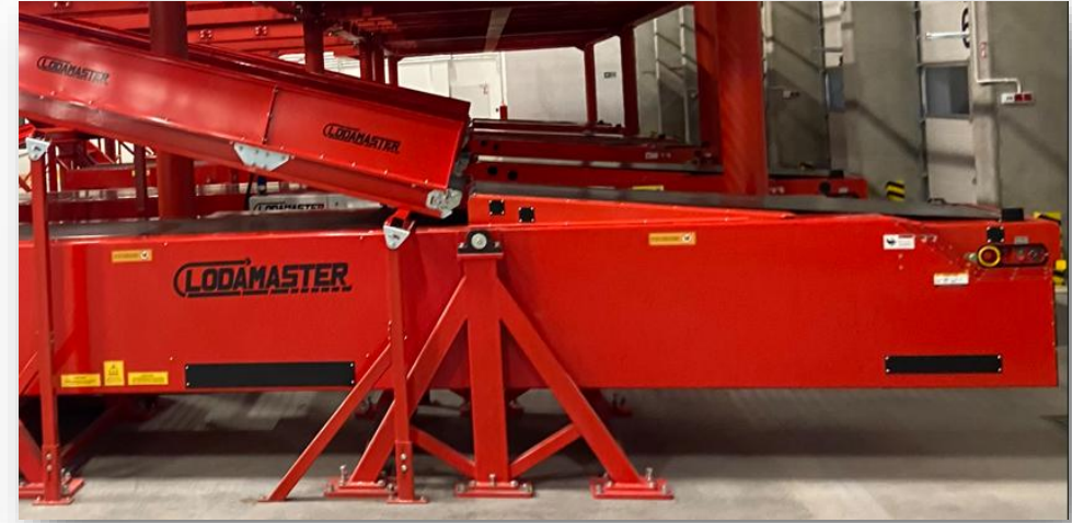
Raised Belt/Sliding Hood
